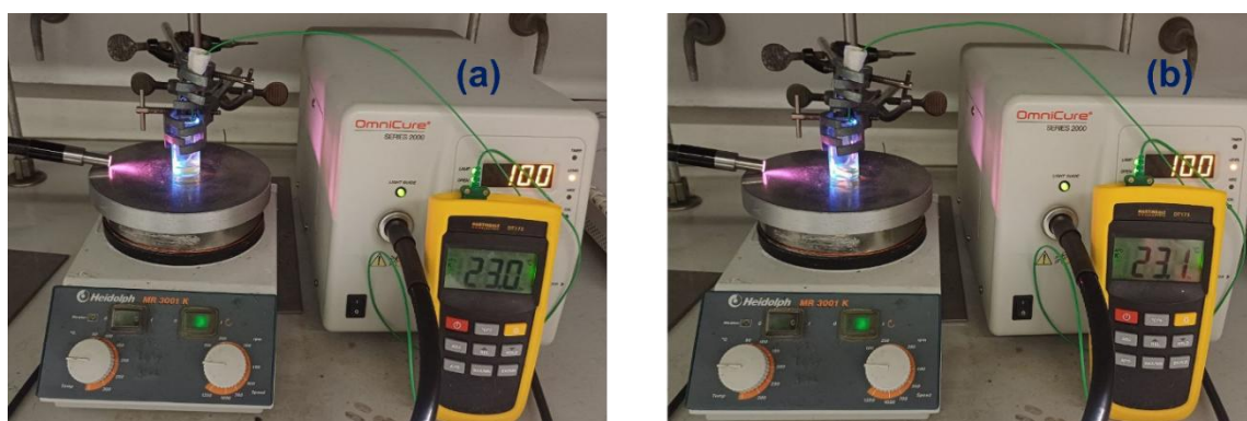
Figure S17. Photopolymerization apparatus, featuring an Omnicure series 2000, 200 W system integrated with a thermostat unit, (a) at the beginning ; (b) after 24 h of reaction
