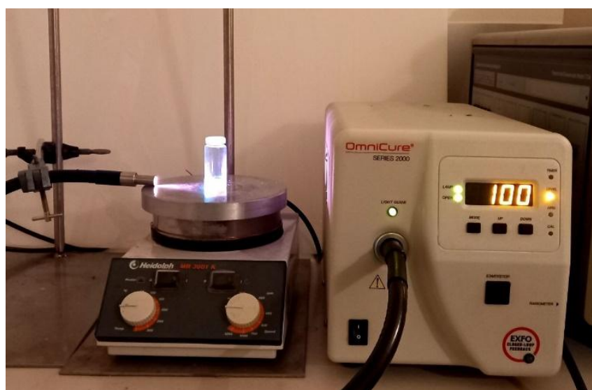
Figure S16. Photopolymerization setup using Omnicure series 2000, 200 W.
